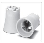
E40 lampholders Casing: porcelain, white, T270 Fixing brackets with slots for screws M5 Weight: 240 g, unit: 48 pcs. Type: 12510/12511 **Ref. No.: 533952 Ref. No.: 533953** with lamp safety catch
